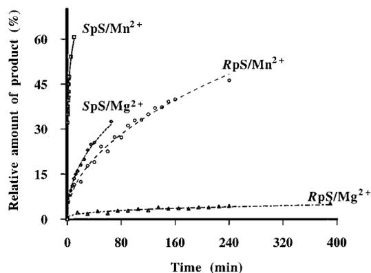
**Figure 2.** Time courses of hammerhead ribozyme-catalyzed reactions. Reactions were performed in the presence of either  $Mg^{2+}$  or  $Mn^{2+}$  ions, with the RpS or the SpS substrate, in which either the *pro-Rp* or the *pro-Sp* oxygen at the cleavage site had been replaced by sulfur (the autoradiograms for ribozyme-mediated cleavage of reactions used in Figure 2 are available as supporting information).<sup>30</sup>
